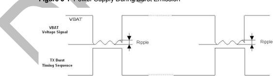
Figure 5-1 Power Supply During Burst Emission
